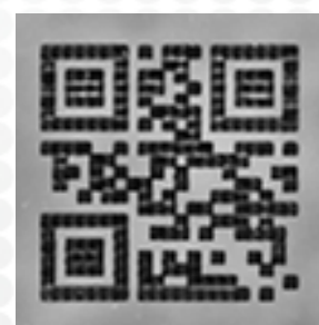
Micro QRcode ( 750\mu\text{m} \times 750\mu\text{m} )
